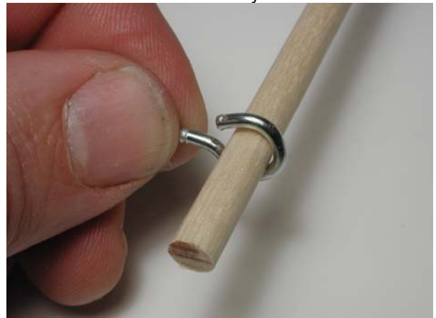
7. Test the dowel in the screw eye for fit. It should be loose, but with little play. Resize the screw eye as necessary.
